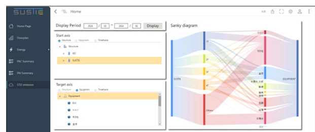
Sankey visualization chart showing energy and CO2 consumption by floors and equipment, highlighting key contributors for targeted optimization
