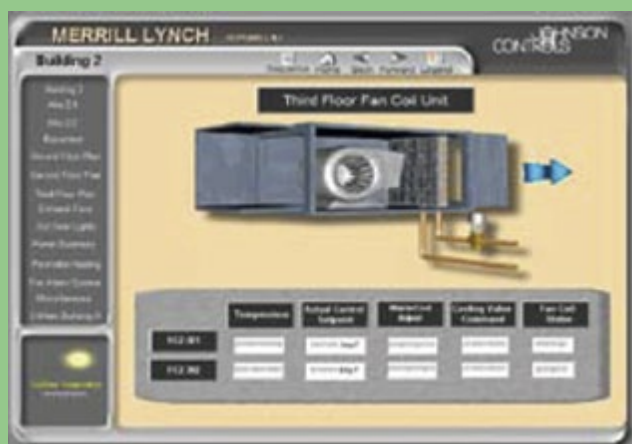
Fan Coil Unit Control in a Merrill Lynch Building
