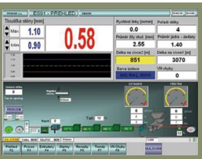
Main Control Screen at PRAKAB a.s.
