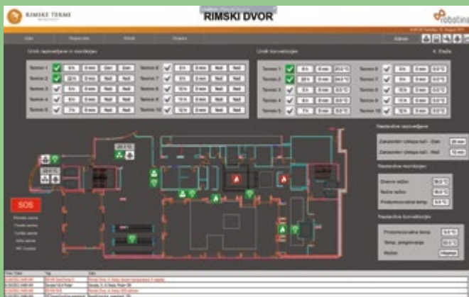
Lighting and Fan Scheduling per Floor of the Resort
