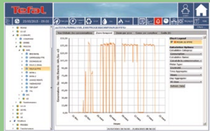
Overall Consumption View of Plant.
