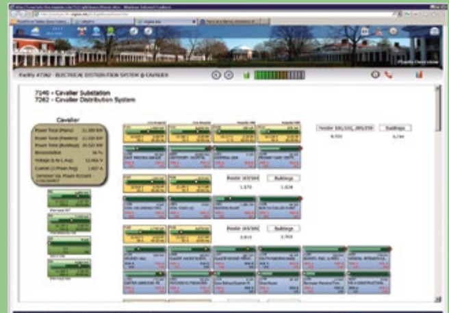
Substation Real-time Reconciliation Screen
