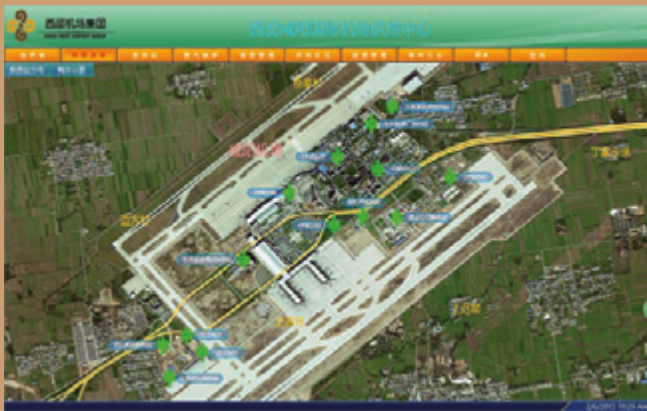
Heat Station Control Using EarthWorX™ GEO SCADA
